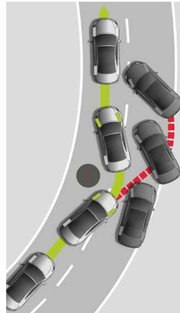
The Electronic Stability Programme reacts to critical driving situations in milliseconds by targeting brake and engine management systems, controlling the speed of individual wheels and bringing the vehicle under control.
